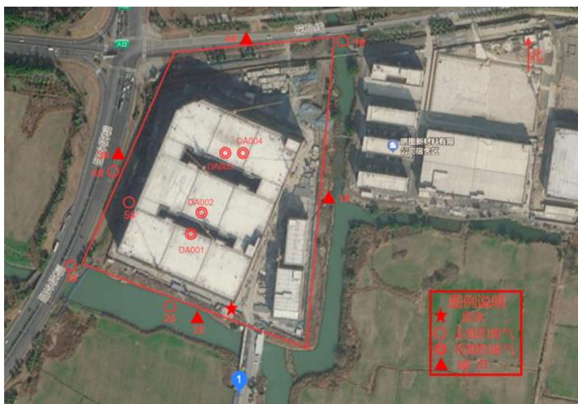
图3.1-4 废气监控点和厂界环境噪声测点布置
